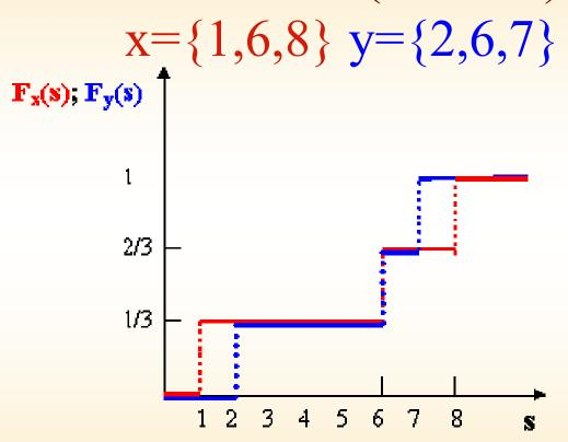
$F_y(s)$  SSD  $F_x(s)$ : Note that the <u>cumulative</u> area below the cdf of y is at every point lower or equal than that of x.
